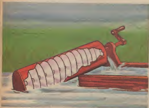
Cutaway view of Archimedes' screw.
